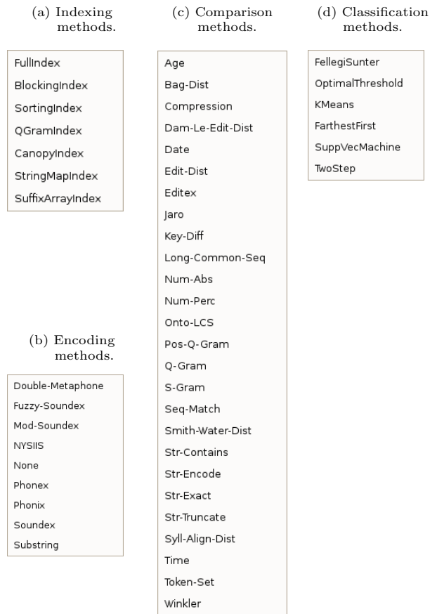
Figure 7: Available methods for indexing (a), string encoding (b), field comparison (c), and weight vector classification (d). These are the pull-down menus from the corresponding Febrl GUI pages.
