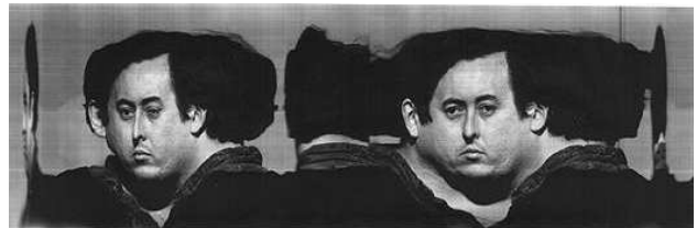
Figure 4: A strip camera image showing a head from all sides taken from Davidhazy (2001)
